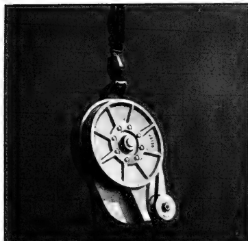
Fig. 1 - Hydraulic power block for hauling crab pots and long-line gear.
